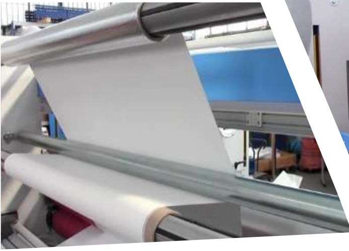
Unwinder and rewriter for coating and liner removing
