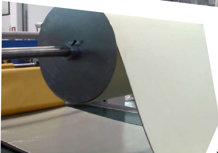
Intermediate unwinder between first and second calander
