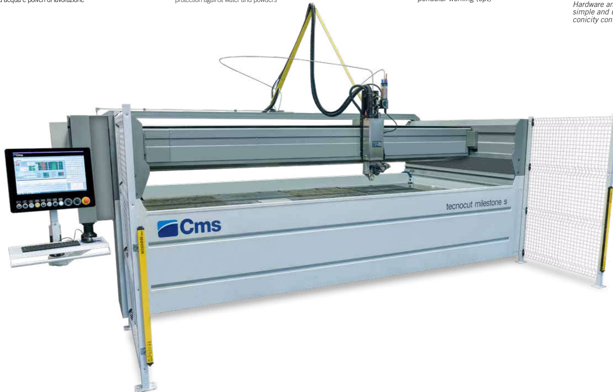
Double cutting table solution for pendular working (opt)
