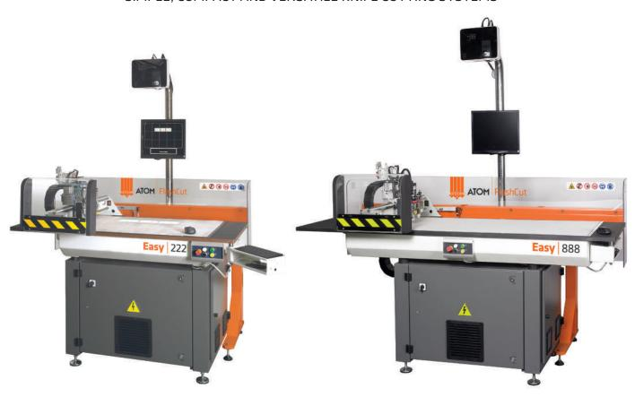
The FlashCut **Easy 222** and **Easy 888** perfectly meet the requests of footwear and leather goods industry. They represent the perfect choice for sample departments and small production batches. Their easy handling, flexibility and cutting accuracy are appreciated also for bigger productions. They can cut leather and hard leather for soles, as well as many man-made materials. Easy to use, they are the best choice for small companies or those who want to automate the cutting process.
