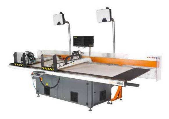
The wide working area together with two independent cutting heads make the **FlashCut Easy 888 L35** a mass production cutting system. Thanks to its ergonomic design, its double working area and friendly use, this model is extremely efficient for cutting a wide material range: soft leather and hard leather for soles. Best solution for footwear and leather goods.
