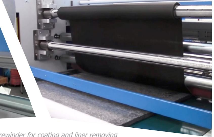
*Unwinder and rewriter for coating and liner removing*
