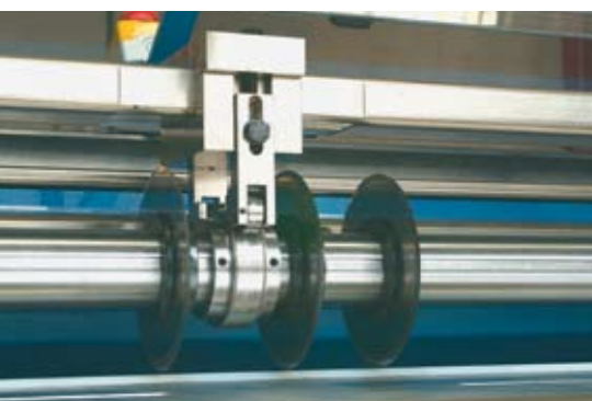
UPPER COUNTER-ROLLER Indispensable accessory for heavy applications.
