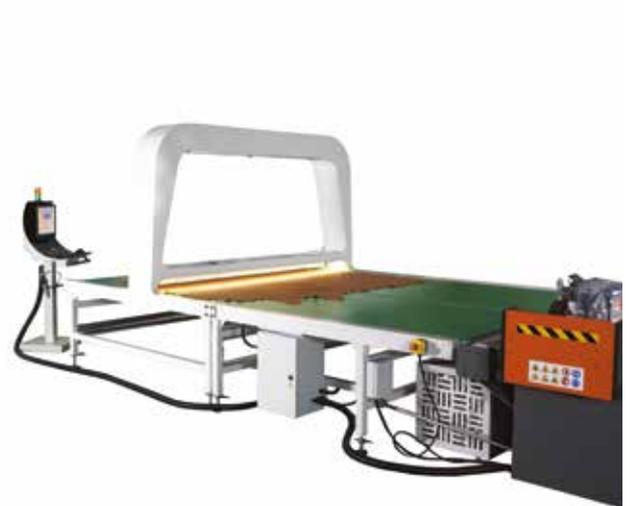
The IntelliView models can automatically acquire leather contour of any kind and colour. The lighting system and the exclusive FlashTracer optical pen allow a clear visualization of the surface and ease the quality area marking.
