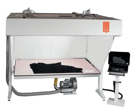
The **Intelliview models**, available both in-line and off-line version, can automatically acquire leather contour of any type and color. The lighting system allows a clear visualization of the surface and it eases the leather inspection.
